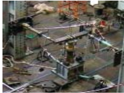
Test rig during coupling tests for axial compression and bending. General view
