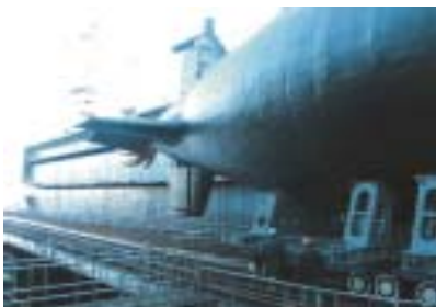
Hydroacoustic coating of the "Saint-Petersburg" submarine
