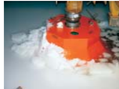
Model tests of a fixed ice-resistant offshore shipping terminal and a tanker in the sea-keeping and ice model tanks
